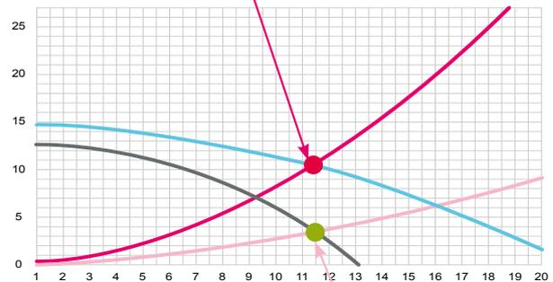
Load loss of an optimised hydraulic circuit in an 8×4 m pool
