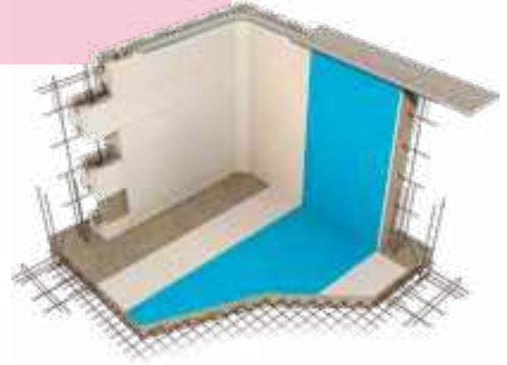
**BLOKIT®SYSTEM POOLS ARE MADE OF REINFORCED CONCRETE.**
